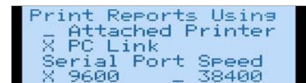
Preferences form on the Q3, showing the settings for printing via the PC
