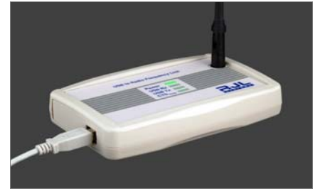
This portion of the RF Link connects to your PC via a USB cable.
