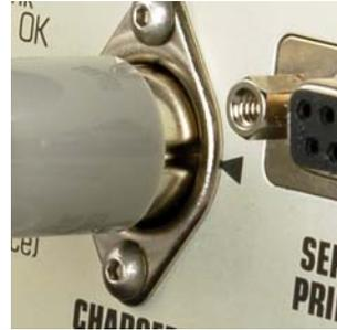
The indentation on the connector must line up with the arrow.
