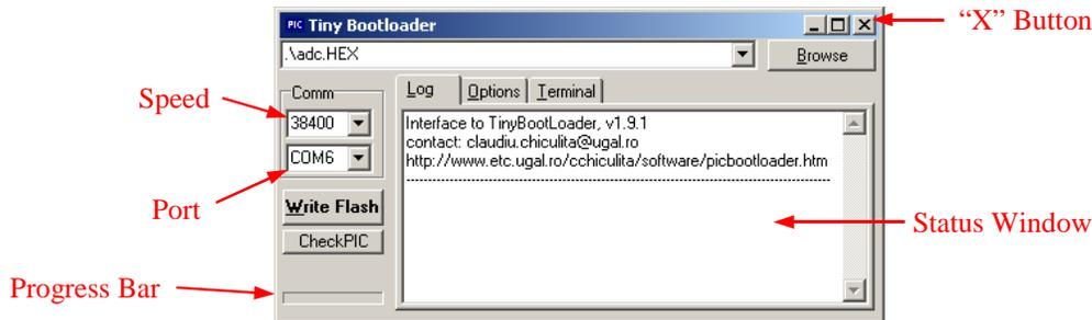
3. Make sure that the speed is set to 38400. Set the port to the same value used by BC. If you are uncertain of which port to use, open BC and select "Configure Serial Port" from the "Options" menu. The port setting will be in the top drop-down box. (Once you have verified which port to use, you **MUST** exit from BC before continuing the firmware update process.
